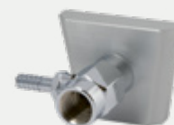
Anodized aluminum wedge for OHMEDA rail clamp bracket, with nipple threaded ISO G. 1/4" F. and hose connector Ø 6 mm (for medical gases) or Ø 7.5 mm (for vacuum).
